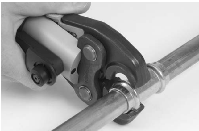
Figure 5 – Opening The Scissor-Style Jaws
