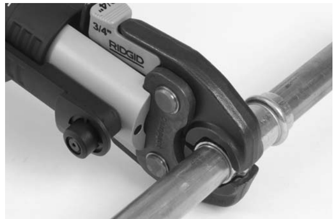
Figure 6 – Placing Scissor-Style Jaw Set Around Fitting
