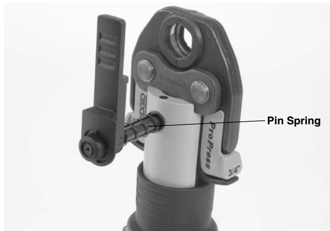
Figure 4 – Fully Open/Unlocked Mounting Pin
