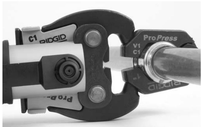
Figure 9 – Attaching Actuator To Press Ring
