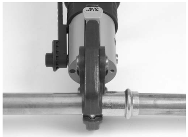
Figure 7 – RP 200-B Tool Square To Tubing
