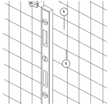
If you were able to locate a wall stud for one or both ends to mount your tissue holder with shelf, drill 1/8" (3mm) holes and mount the mounting bracket with the two screws provided. (Skip to step 4 if both mounting studs were mounted into wall studs.)
