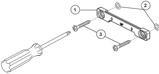
With the mounting bracket (1) oriented as shown, place it over the installed anchors (2) and screws (3).
