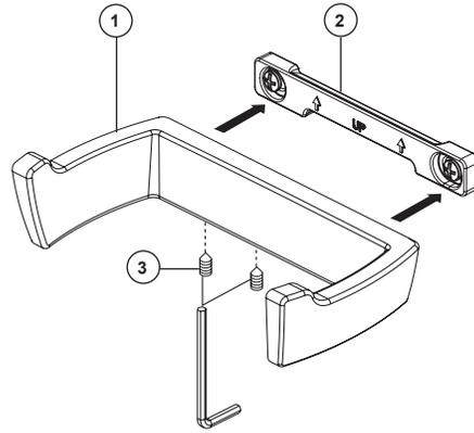
Position robe hook (1) over mounting bracket (2) and tighten set screw (3).
