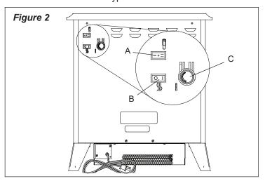
The "=" position is for operating the unit with the provided remote control. When in "=" position the unit is operated with the ON and OFF buttons of the remote control.
