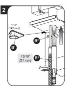
For countertop thicknesses less than 1/16" thick use the flange (B1), for all other installations use the metal washer (B2).
