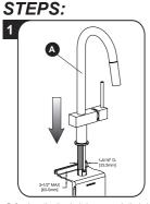
Before inserting the single lever group in the hole of the sink, make sure that the base gasket is properly positioned in its seat and that the flexible hoses are well tightened to the body of the tap. Place the single lever group in the hole of the sink,
