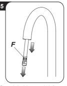
Remove the hand shower, completely disconnected, to carry out the replacement (F). Finally reassemble the whole with the opposite procedure.
