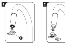
Before removing the aerator make sure that the faucet is turned off. Unscrew the aerator using the aerator installition key (E) included with the faucet if the aerator is clogged just rinse it with running water. Do not use detergents. Reassemble the aerator by following the instructions in reverse order.
