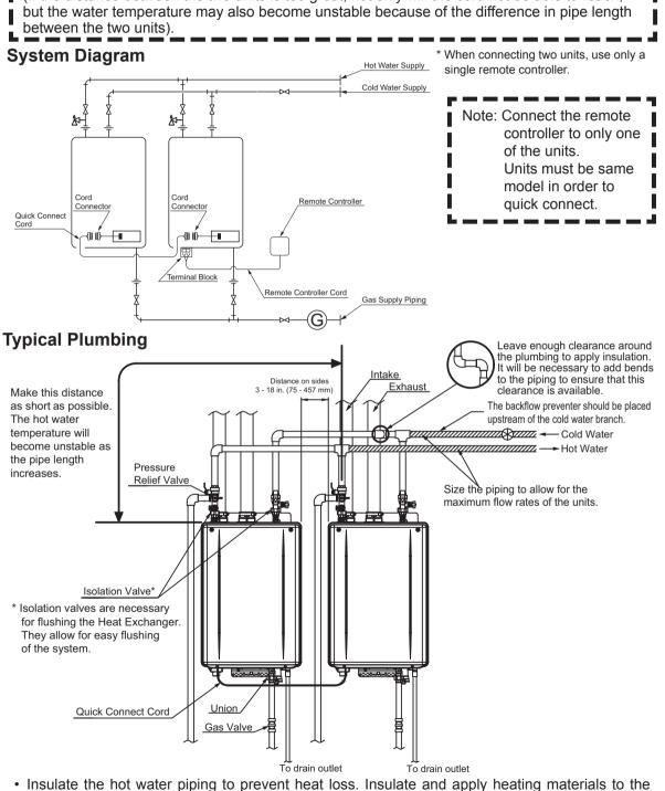
cold water supply piping to prevent heat loss and freezing of pipes when exposed to excessively
