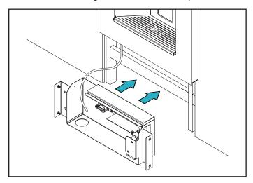
3. Using four #8 flathead screws, start the screws to hold the unit in place.
