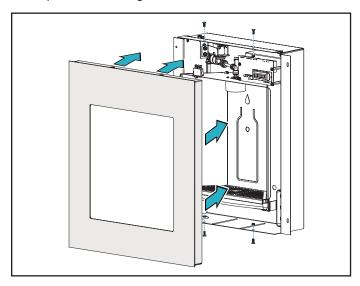
**NOTICE**Attach the front cover with the top two mounting screws to prevent it from falling away from the water dispenser while the filter unit is being installed.
