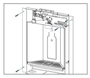
4. Locate the electrical gang box, at the lower right-hand corner of the water dispenser, and remove the cover.
