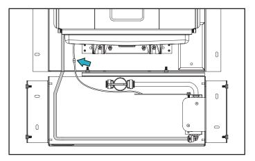
8. Connect the 1/4" tube to the fitting below the filter, as shown.
