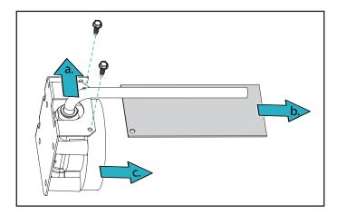
d. Screw the bracket to a wall stud, then reassemble the filter head, NFC card, and inlet water tube.
