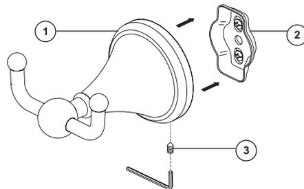
Position robe hook (1) over mounting stud (2) and tighten set screw (3).
