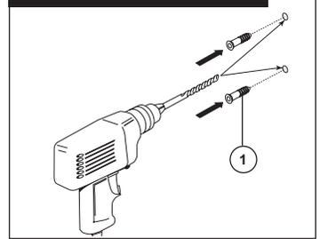
If you were able to locate a wall stud to mount your accessory, drill 1/8" (3mm) holes and mount the mounting stud with the two screws provided. (Skip to step 4).
