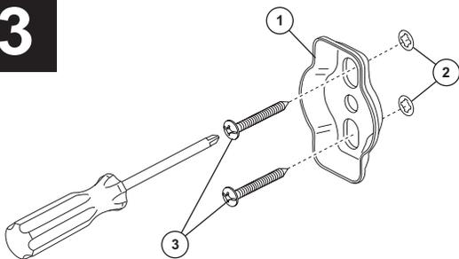
With the mounting stud (1) oriented as shown, place it over the installed anchors (2) making sure the notch on the post points downward and install screws (3).
