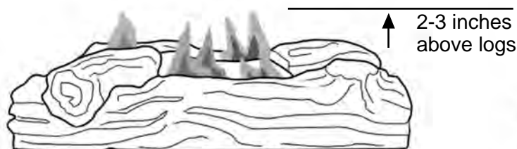
Fig. 22 - Correct Burner Flame Pattern
