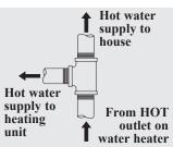
Tee fitting for vertical hot water supply lines.
