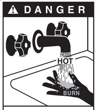
Water temperature over 125° F can cause severe burns instantly or death from scalds.
