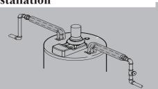
**Typical horizontal piping arrangement** Please install the insulation, according to the illustrations above, that best meets your requirements.
