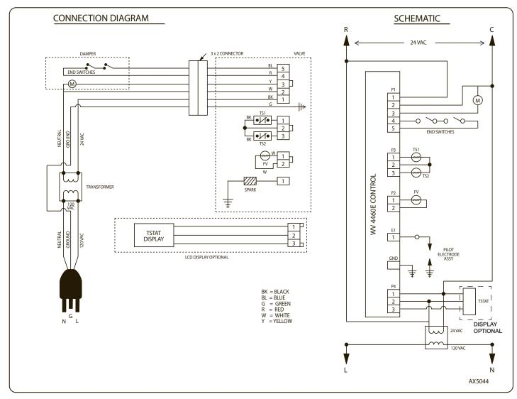
**A**CAUTION! Label all wires prior to disconnection when servicing controls. Wiring errors can cause improper and dangerous operation. VERIFY PROPER OPERATION AFTER SERVICING!
