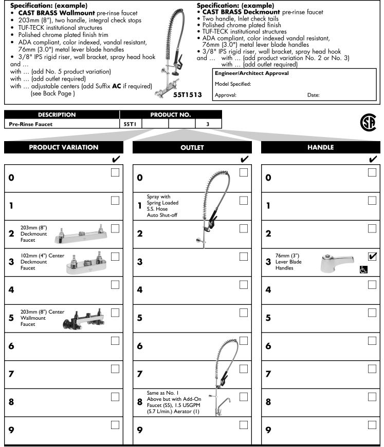
(1) See Page 9.C.2 for **Optional Swing Spouts**. These spouts can ONLY be added to **Outlet Option No. 8**, and **55T1090**. Refer to www.specselectonline.com for individual models.
