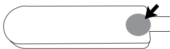
Fig. Apply a small area of thermal compound to the back of the sensor case where shown
