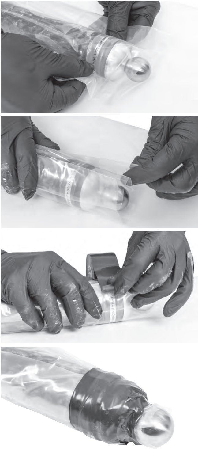
Figure 14 – Folding Sleeve Around Packer and Taping
