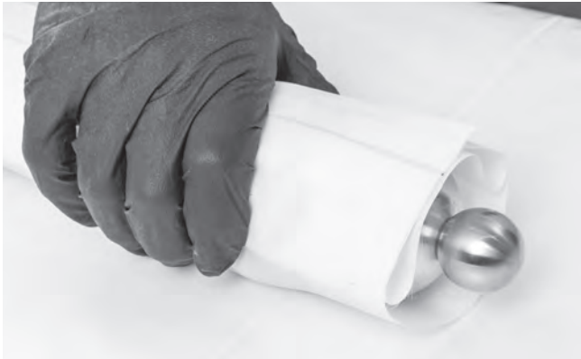
Figure 21 – Folding Containment Tube Around Packer
