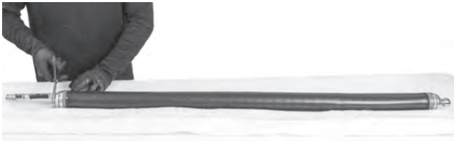
Figure 25 – Measuring Containment Liner
