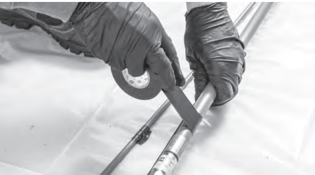
Figure 8 – Marking Patch Position On Camera Push Rod, Transferring To Air Push Rod or Air Hose
