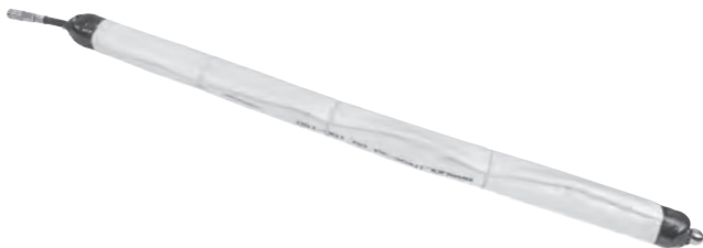
Figure 26 – Packer With Liner, Ends Taped, Doubled Over Elastic Bands Applied Every 12"
