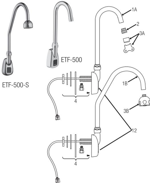
†† TO MOUNT FAUCET ON A SURFACE BETWEEN 0.41" (10 MM) AND 1.00" (25 MM) THICK, USE THE HARDWARE SHOWN BELOW.
