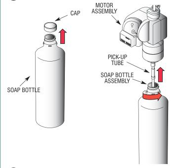
Slide Soap Assembly up over Straight Tube and fit into the Motor Assembly. Twist Soap Assembly clockwise to lock into place.
