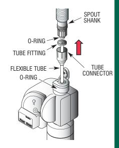
Screw Tube Connector onto Spout Shank and tighten.
