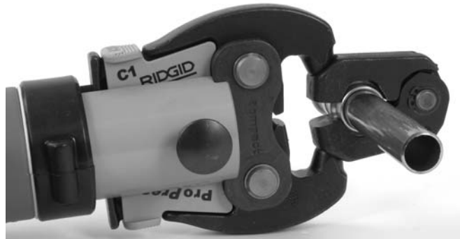
Figure 10 – Attaching Actuator To Press Ring
