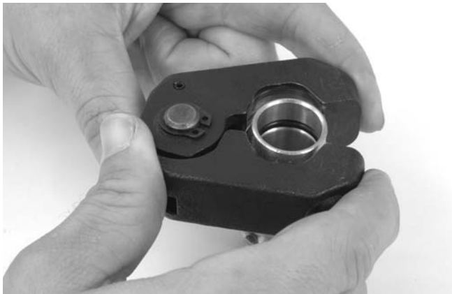
Figure 9 – Installing Press Ring Onto Fitting
