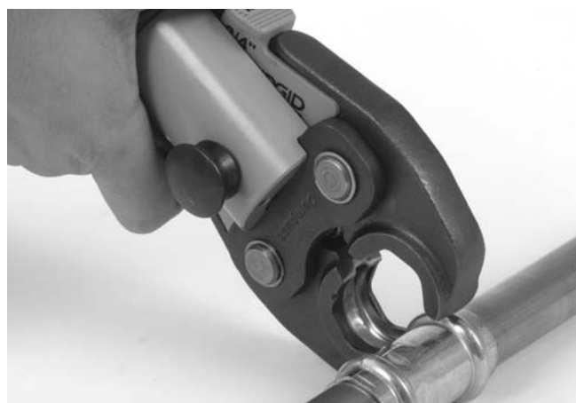
Figure 6 – Opening The Scissor-Style Jaws
