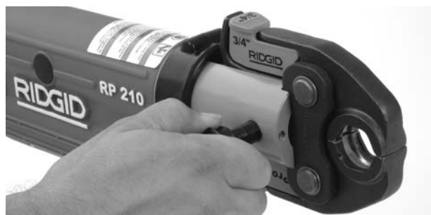
Figure 4 – Fully Open Attachment Mounting Pin
