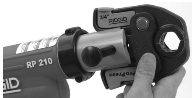
Figure 5 – Slide Attachment Into Tool
