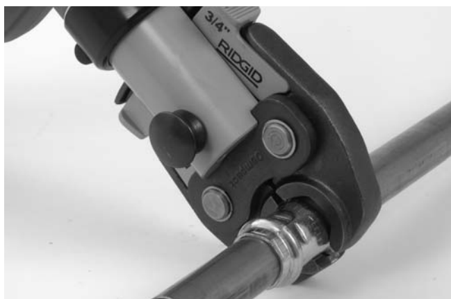
Figure 7 – Placing Scissor-Style Jaw Set Around Fitting
