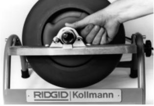
Figure 3 – Locking Front Bracket
