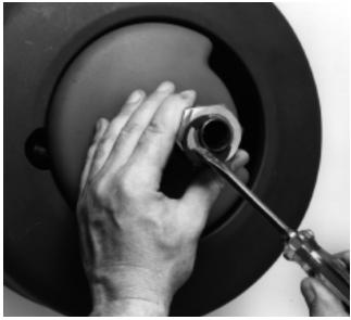
Figure 14 – Removing E-Clips
