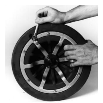
Figure 12 – Loosen Cable Bracket
