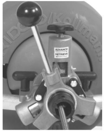
Figure 9 – Autofeed in Reverse Position
