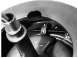
Figure 16 – Position New Cable Under Bracket
