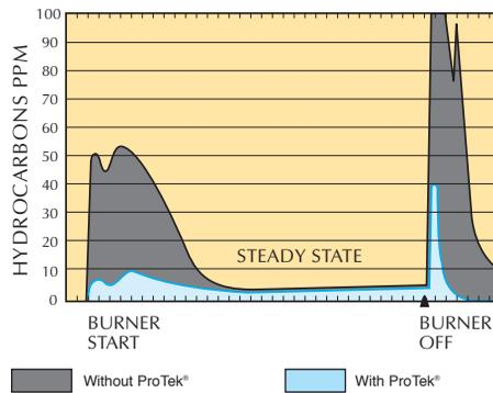
Hydrocarbon emissions are greatly reduced when the Delavan ProTek® Nozzle System is used. Hydrocarbons are typically elevated at start-up and shut-down of the nozzle firing, as both of these graphs show. When the ProTek Nozzle System is installed, the dramatic benefits are seen in these charts which show comparative results with and without the ProTek® valve. Results will vary by application.
