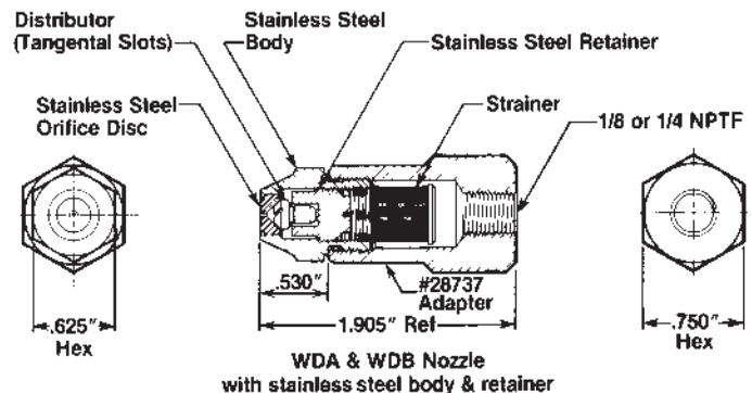
WDA & WDB Nozzle with stainless steel body & retainer
