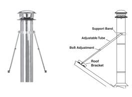
A Roof Brace Kit can be used whenever there is a need to stabilize the chimney above the roof level. The Roof Brace Kit should be used at a midpoint on the chimney. Braces adjust from 4' to 7-1/2'.
