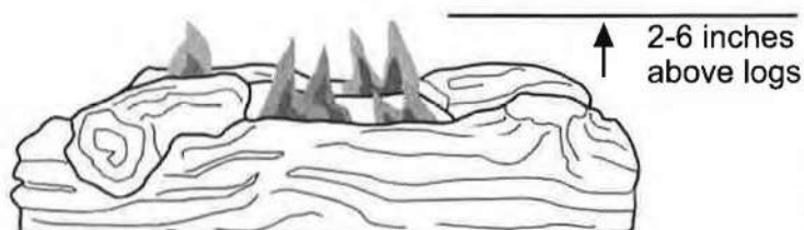
Fig. 29 - Correct/Normal Flame Pattern with short flames
