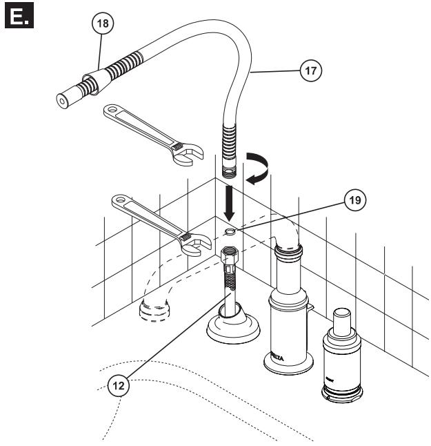
**E.** Slide hose (17) through conical nut (18). Attach hose (17) to braided hose (12) using gasket (19) and tighten. DO NOT install hand shower yet.
