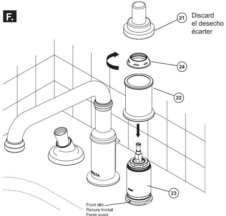
**F.** Remove the cap (21) from the valve body (23) and discard. Slide sleeve (22) on valve body (23), aligning it to the front slot and push down till flush with deck. Thread bonnet cap (24) on valve body (23) clockwise, hand tight.
