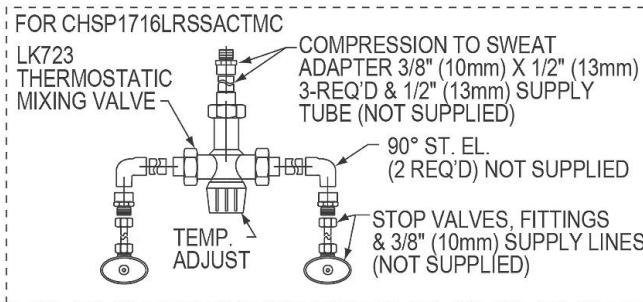
NOTE: USE TEFLOON TAPE FOR ALL WATER CONNECTIONS. DO NOT USE PIPE DOPE.
