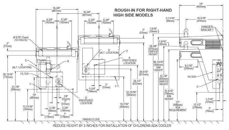
A = Recommended water supply location. Shut off valve (not furnished) to accept 3/8" O.D. unplated copper tube. 3" (76mm) maximum out from wall. B = Recommended location for waste outlet 1-1/2" O.D. drain. Drain stub 2" (51mm) out from wall.
