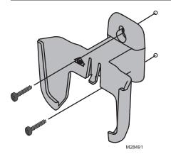
Mount the sensor on a vertical exterior wall, at least 6 inches below any overhang. Choose a location protected from direct sunlight.
