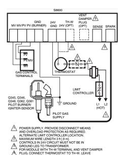
Fig. 8. Typical wiring connections for 24 volt control in intermittent ignition system with \$8600.
