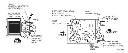
Fig. 6. Top view of gas control.
