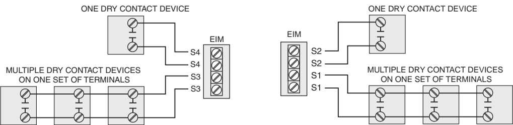
Fig. 187. Wiring dry contact devices.
