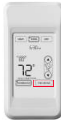
Fig. 313. Reading temperature at the Portable Comfort Control.
