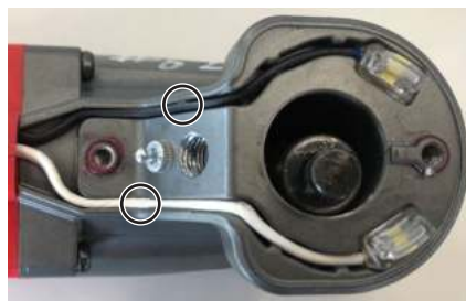
Place white and black wire in corresponding wire traps.
