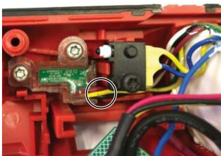
Place FUEL gauge wire into wire trap.
