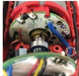
Visually check that Blue wire is free from Rotor.
