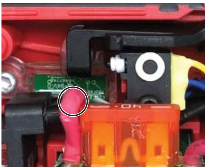
Wrap red wire as shown to avoid interference with slide button.
