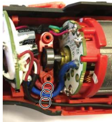
Place red, blue, and black wire in corresponding wire traps.
