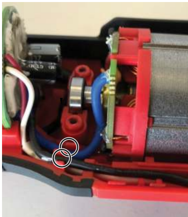
Insert white in trap before Black wire.
