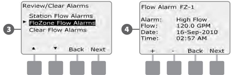
Note each station which has an alarm, then See Clear Flow Alarms in this section for more details on how to clear flow alarms.
