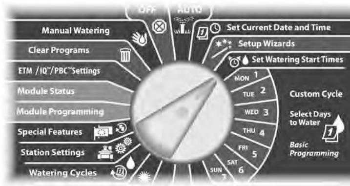
**1** The Set Start Times screen appears. Press the + and – buttons to set Start Time for the current program; then press Next.
