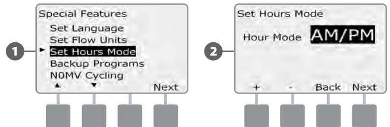
! **NOTE:** Auto defaults to AM/PM when 60 Hz power is detected and to 24 Hour mode when 50 Hz power is detected.
