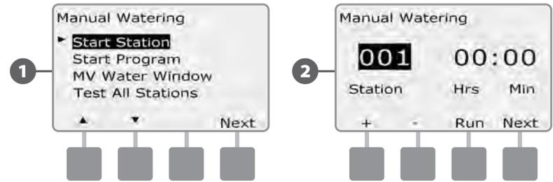
**3** The Station Run Time will default to the Program Run Time. Press the + and – buttons to adjust the station Run Time (from 0 hours, 1 minute to 12:00 hours). Press the Run button to start irrigation for that station.
