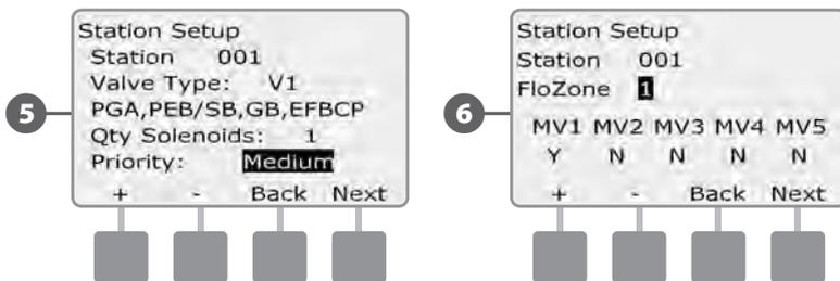
**NOTE:** If you have already set up your MVs and FloZones, the MV assignments for the currently selected FloZone will be shown in the bottom portion of the screen.
