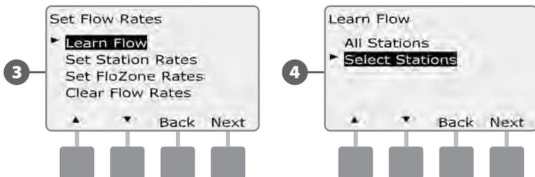
5 Press the Yes and No buttons to select the stations you would like to include. Press Next and Back buttons to select stations; then press Next.
