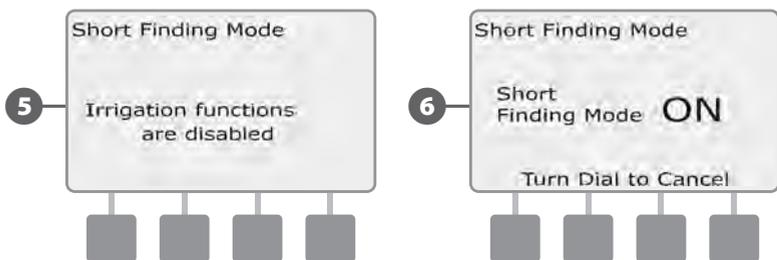
**!** **NOTE:** Use a clamp meter to isolate and repair shorts in the two-wire path. Once repairs are finished, be sure to return to the controller and turn the dial to exit short finding mode. Irrigation can not occur until short finding mode has been cancelled.
