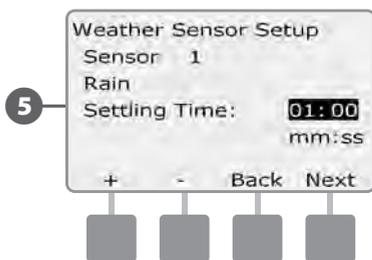
**NOTE:** Settling time is how long a weather condition must last before the controller takes action. For example, if a freeze sensor has a 5 minute settling time then the temperature would have to remain below the sensor's threshold set point for 5 minutes before irrigation is paused. Settling time can be set for immediate (0 seconds) or up to 10 minutes long.
