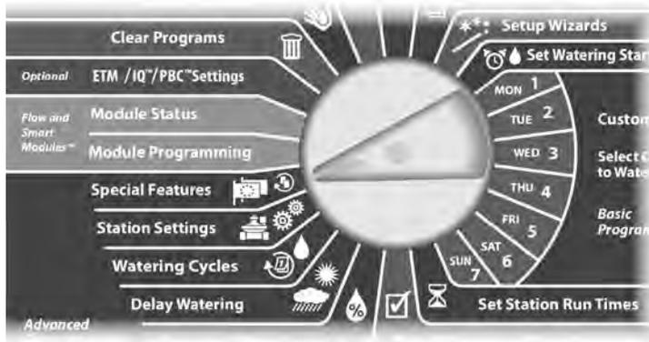
1 The Special Features screen appears. Press the Down Arrow button to select NOMV Cycling; then press Next.
