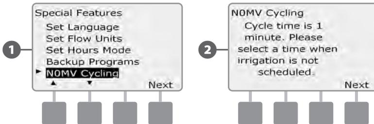
3 The NOMV Cycling screen appears. Press the + and - buttons to set the desired time for cycling to start; then press Next.
