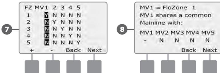
**↻** Repeat this process to set up additional master valves. Be sure to note each MV on your Programming Guide for future reference.
