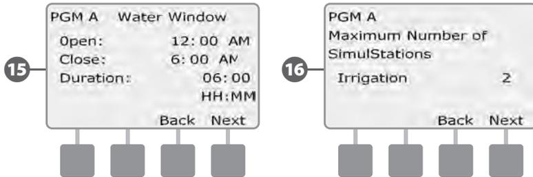
**17** The Maximum Number of SimulStations for controller review screen appears with the maximum number of stations that can operate simultaneously for that controller are displayed. Press Next.
