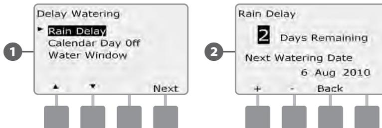
**NOTE:** A Rain Delay affects all programs, but stations set up as Non-irrigation will still run during a Rain Delay.
