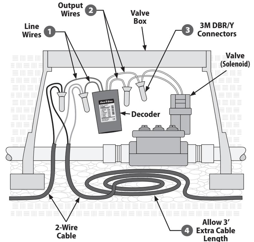
Typical Field Decoder Wiring
