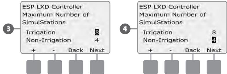
**NOTE:** The Non-Irrigation SimulStations setting is used to configure the maximum number of Non-Irrigation stations that can operate simultaneously and allows you to balance the number of Irrigation and Non-Irrigation stations that can operate simultaneously. Also note that when SimulStations are set to a maximum of 8, if a Normally Closed Master Valve has to be held open for irrigation to occur, it will limit the maximum number of SimulStations to 7.
