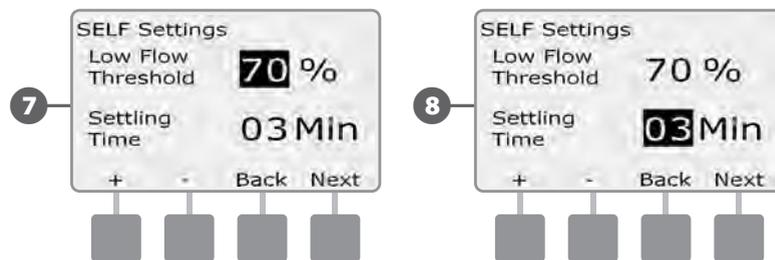
**!** **NOTE:** If you are using Cycle+Soak, be sure to set your SEEF and SELF settling times shorter than the cycle portion of your Cycle+Soak station runtimes. A SEEF or SELF condition can not be detected if the SEEF and SELF settling times are equal to or longer than station cycle times.
