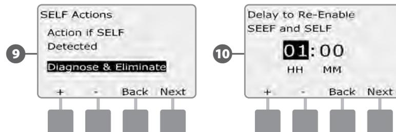
11 Press the + and – buttons to set minutes before Re-Enable; then press Next.
