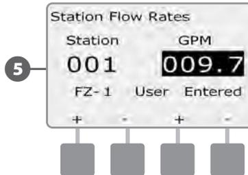
Repeat this process to manually set up Flow Rates for additional stations as desired.
