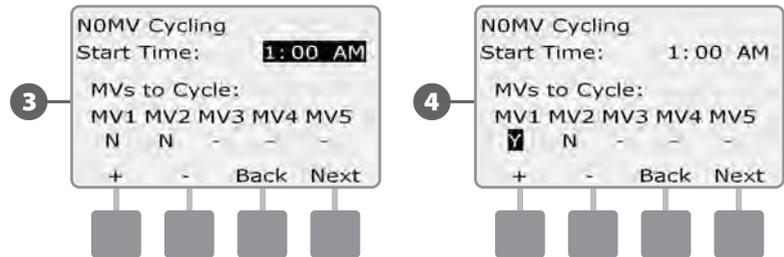
5 Press the Next and Back buttons to navigate through the MVs and repeat the selection process as desired.
