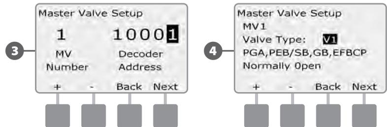
**NOTE:** Rain Bird residential valves (DV and JTV series) are not compatible with ESP-LXD decoders. Use Rain Bird commercial valves (PGA, PEB, GB, EFB-CP and BPE series).
