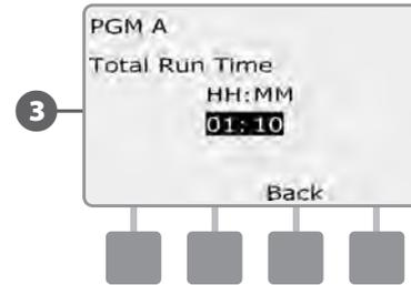
**NOTE:** For stations set up for Cycle+Soak, the Cycle Time (when irrigation is occurring) will be included in Program Run Time calculations but Soak times will NOT be included. See Section D, Cycle+Soak, for more details.
