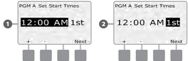
Change the Program Select switch and repeat this process to set up additional Watering Start Times for other programs as desired.
