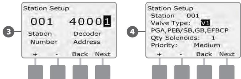
**NOTE:** Station Priorities are only used when Station Sequencing is set to Sequence by Station Priority. If you're using the default Sequence by Station Numbers, then skip the next step by pressing Next.
