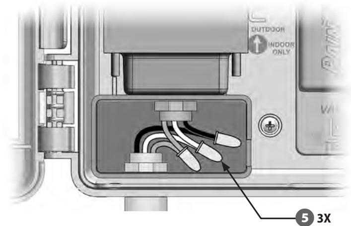
**⚡ WARNING:** The ground wire **MUST** be connected to provide electrical surge protection. You will void the controller warranty if you do not ground the controller.
