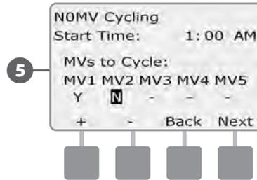
**NOTE:** There is no need to cycle Normally Closed Master Valves (NCMV) open, so they are not included in the selection screen. NCMVs will show as - and can not be changed.
