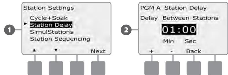
Change the Program Select switch and repeat this process to set Station Delay for other programs as desired.
