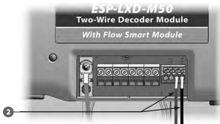
**!** **NOTE:** If your weather sensor requires 24V power from the controller, the connectors to the left of the sensor and common connectors can be used.
