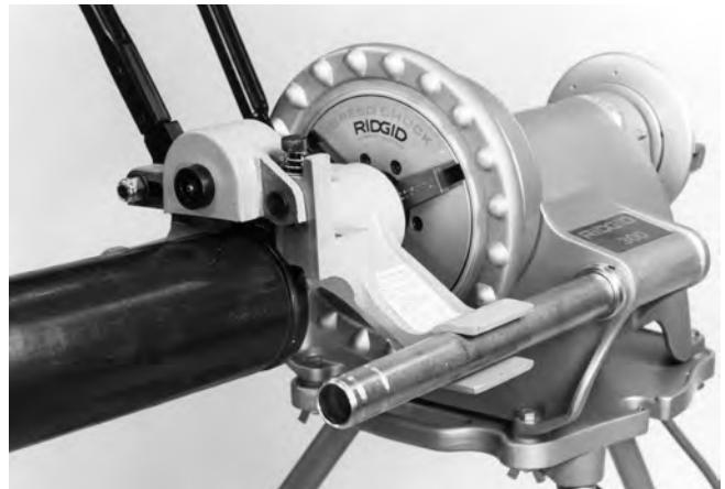
Figure 9 – Feed Handle in UP Position
