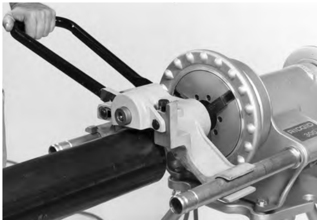
Figure 12 – Forming the Roll Groove
