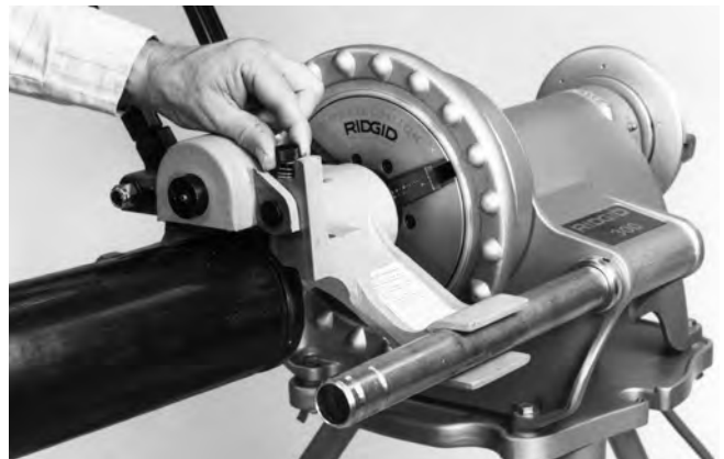
Figure 10 – Loosen Depth Adjustment Screw
